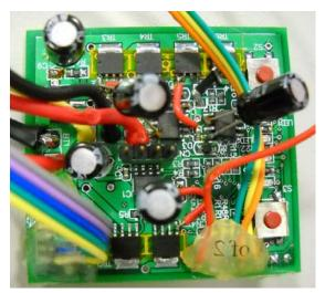
Figure 6-1 Main board of the controller
